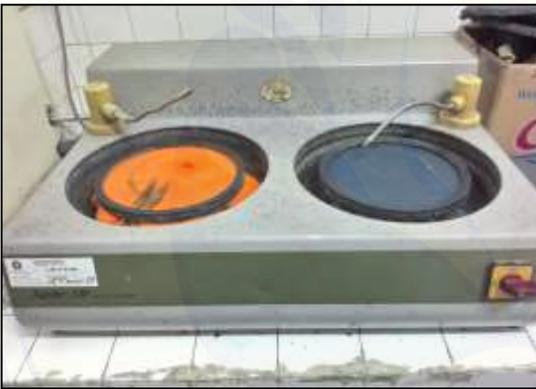
Mesin *Grinding Polishing*
