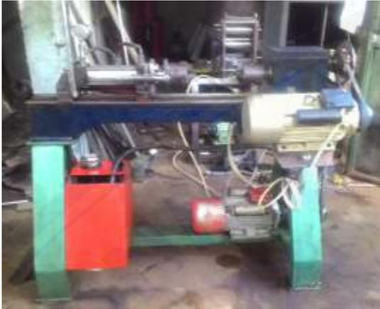
Mesin *Friction Welding*
