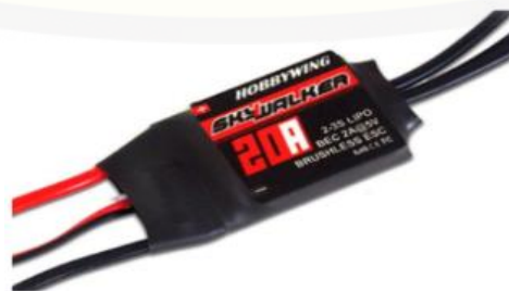
Gambar 3.6 ESC Hobbywing Skywalker 20 A
