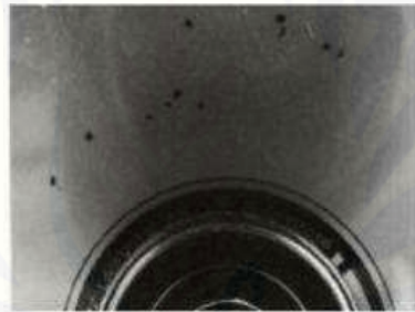
Gambar 2.17 Cacat Black Dots (Anonymous, 2014)
