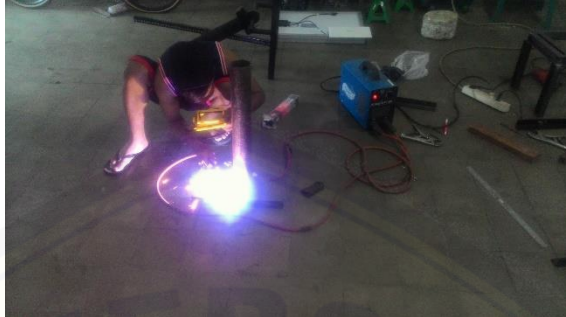
Gambar C.1 Proses Pengelasan Rangka Panel Surya
