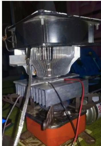
Gambar 3.5 Prototype pengujian modul TEG TE-MOD-10W4V-40
