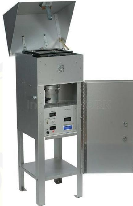
Gambar 3.2 Unit High Volume Air Sampler (HVAS)
