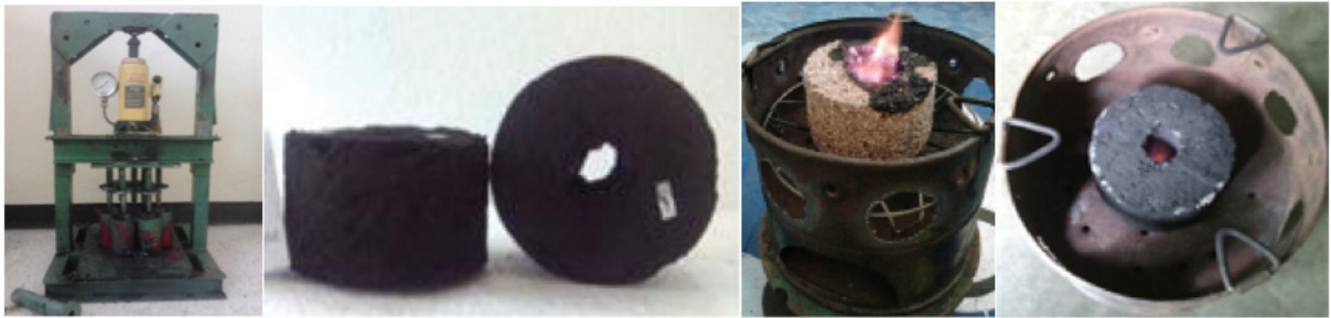
Figure 9 (a) A hand use of briquette pressing for producing briquette (b), the colour flame of briquette red first (c) turning to blue (d).
