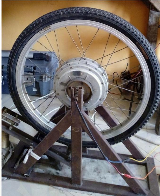
Gambar 3.11 Motor listrik DC magnet permanen
