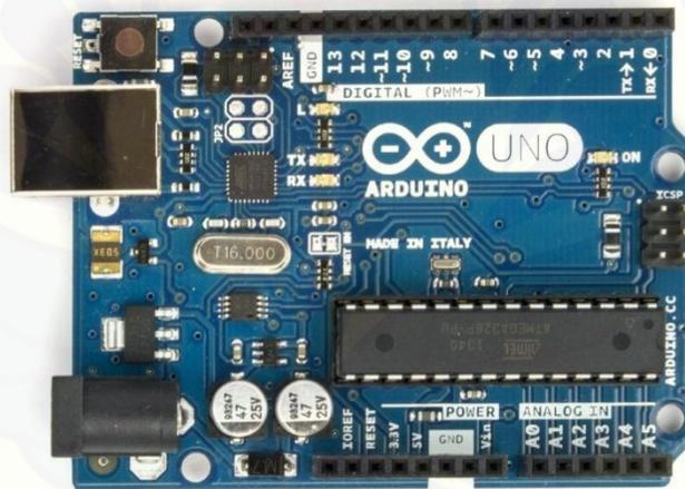
Gambar 2.20 *Board* Arduino Uno
