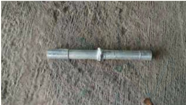
Hasil pengelasan friction welding Al6061
