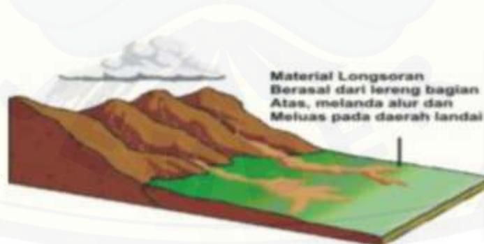
Gambar 2.5 Rayapan Tanah
