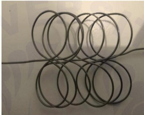
Gambar 3.1 Profil *double helical* pipa kapiler
