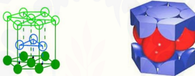
Gambar 2.4 Struktur Kristal Hexagonal Closed Packed (Callister, 2012).
