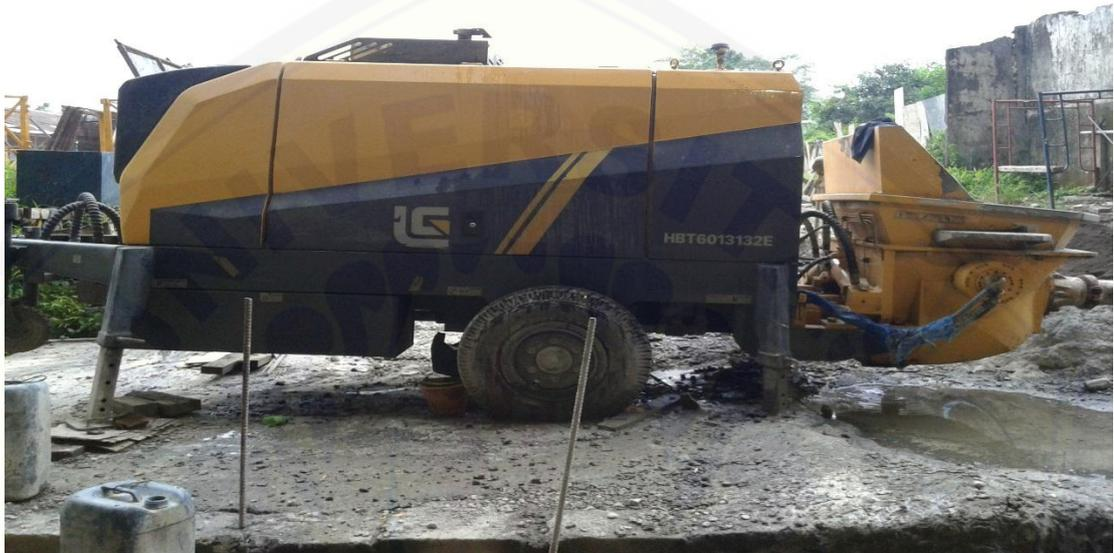
Gambar 1.1 Alat Pompa Kodok
