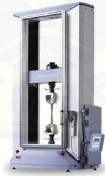
Gambar 3.8 Mesin uji tarik merk Shimadzu Autograph AG-X 5 KN
