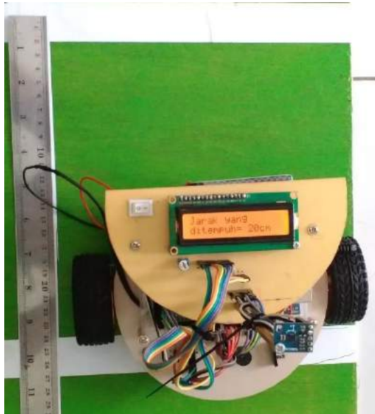
Gambar 3.15 Pengujian Sensor Rotary Encoder
