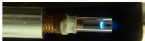
Gambar 3.3 *Meso-scale Combustor*
