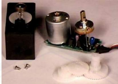
Gambar 2.15 Sistem mekanik motor servo
