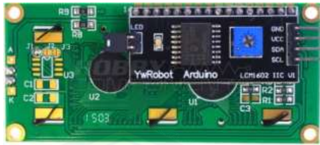
Gambar 2.10 I2C LCD (sumber : http://hobbycomponents.com )
