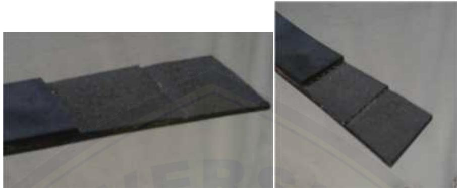
**Gambar 2.11** Foto Makro sambungan *belt conveyor*
