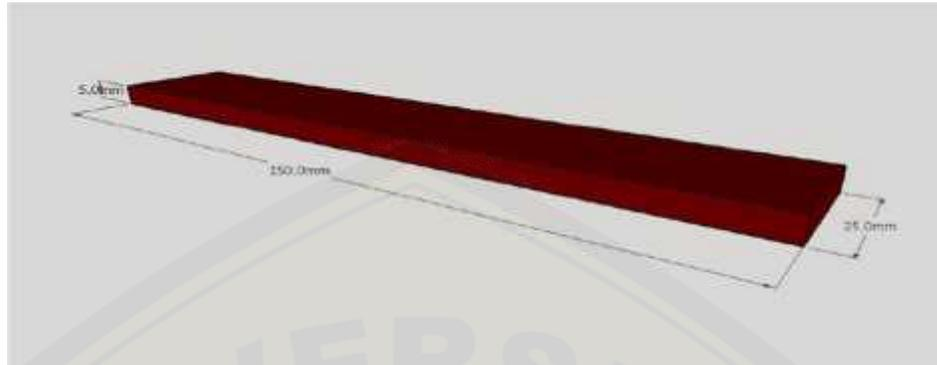
**Gambar 2.13** Standar Sampel Uji ASTM D3039 (Nasiruddin, 2014)
