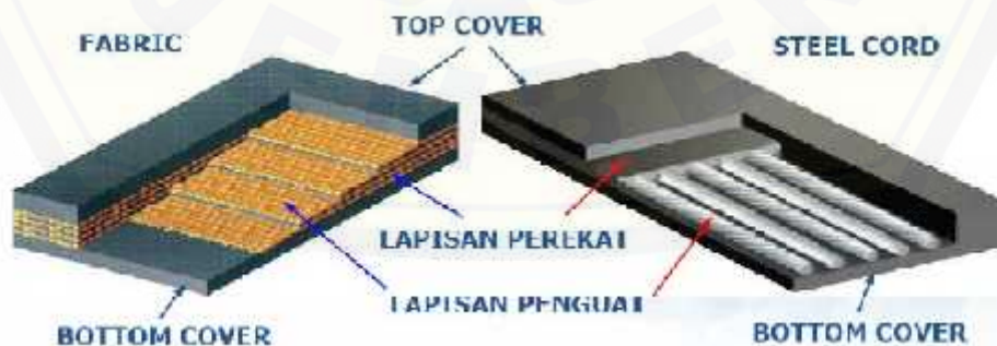
Gambar 2.4 Perbedaan Fabric Belt dan Steel Cord Belt Conveyor
