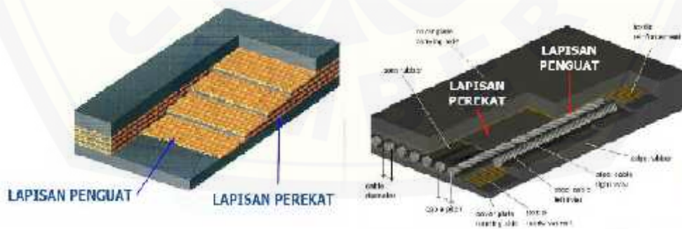
Gambar 2.5 Lapisan Penguat Fabric dan Steel Cord belt .
