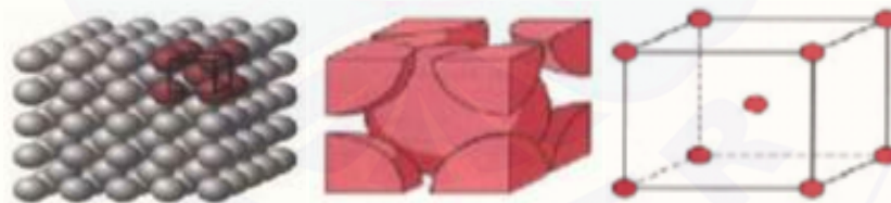
Gambar 2.1 Struktur kristal Body Centered Cubic (BCC) (Mangonon, 1999)
