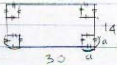
$$V = p \times l \times t \quad \begin{array}{l} 1 \\ -p = 30 - 2a \\ l = 14 - 2a \\ t = a \end{array}$$
