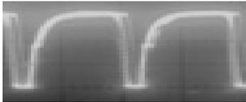
(b) Tigger signals using PWM from driver circuit
