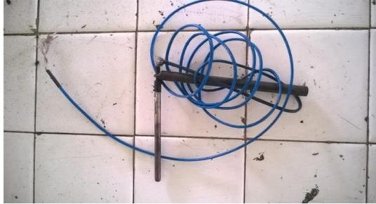
Gambar 3.2 Kabel Termokopel Tipe-K
