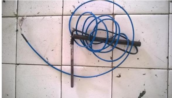
*Gambar 3.2 Kabel Termokopel Tipe-K*
