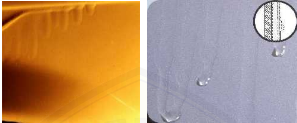
Gambar 2.17 Cacat runs (Sumber: The chemical company BASF , 1990 (online)).
