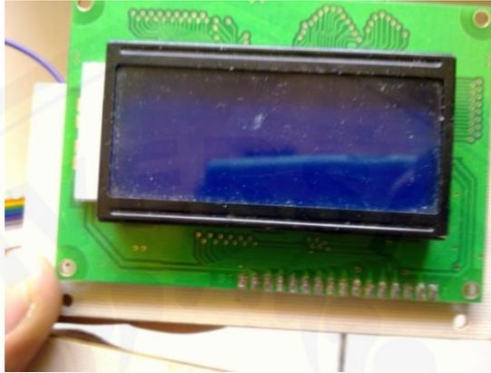
Gambar 3.4 LCD 16 x 4
