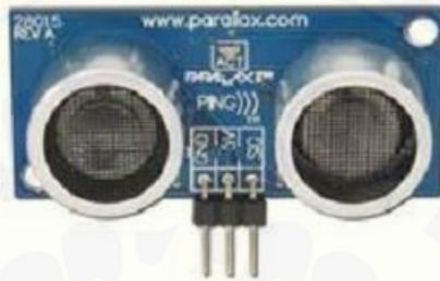
Gambar 2.4 Sensor Ultrasonik Ping
