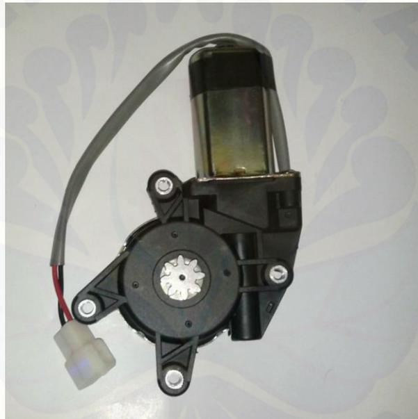
Gambar 2.7 Motor DC (*Power Window*)
