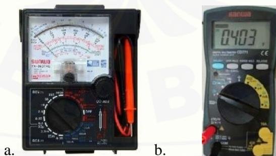
Gambar 2.6 Multimeter (a) Analog; (b) Digital
