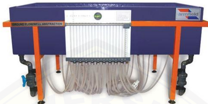
Gambar 3.1 Groundwater Flow and Well Abstraction (sumber: manual instruction Ground Water flow, Wells abstraction unit )
