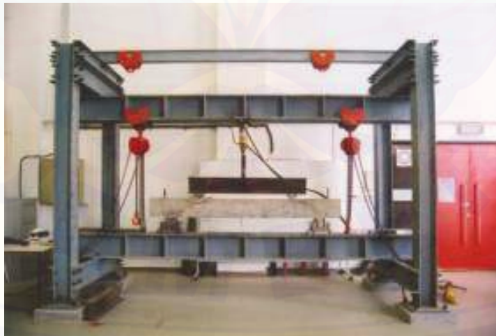
Gambar 2.24 Loading frame (sumber: http://www.fst.umac.mo/en/lab/structure/ )
