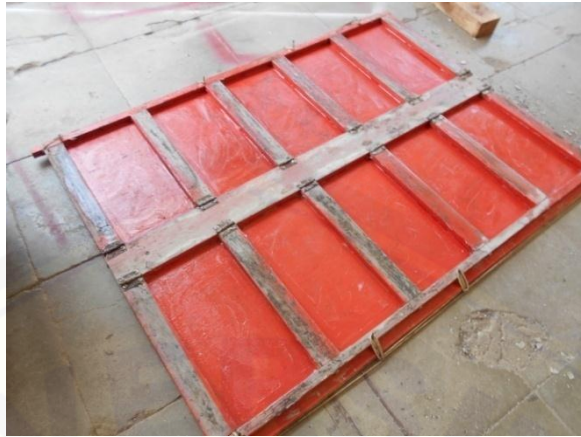
Gambar 4.1 Cetakan Material Wall/flooring
