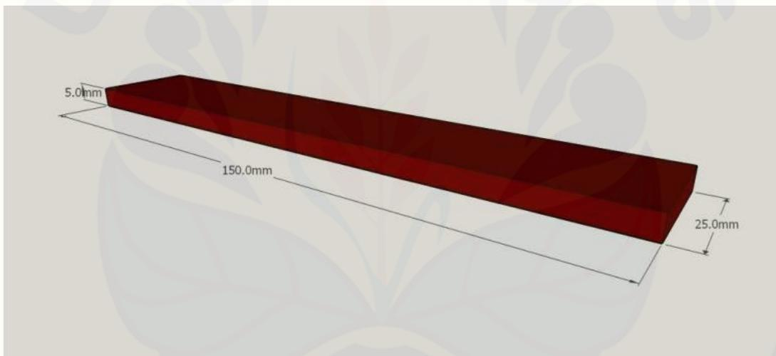
Gambar 2.16 Standar persiapan sampel uji ASTM D 3039.
