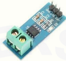
Gambar 4.3 Sensor Arus ACS712-20A-T
