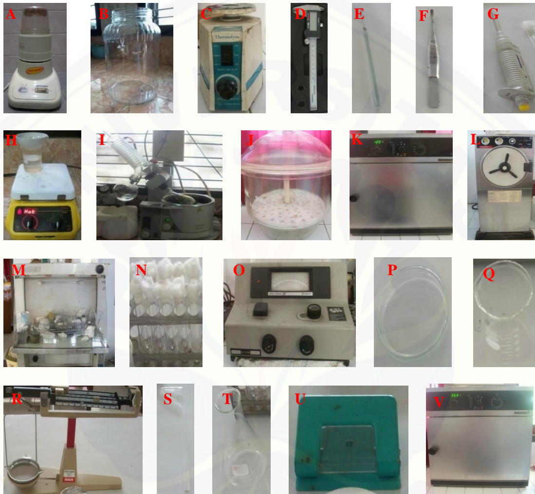
Gambar I.1 Alat Penelitian (A) Blender; (B) Toples kaca; (C) Thermolyne ; (D) Jangka sorong digital; (E) Ose; (F) Pinset; (G) Mikropipet ; (H) Water bath ; (I) Rotary evaporator ; (J) Desikator; (K) Oven; (L) Autoclave ; (M) Laminar flow ; (N) Tabung reaksi; (O) Spektrofotometer; (P) Petridish tidak bersekat; (Q) Gelas ukur; (R) Neraca; (S) Gigaskrin; (T) Tabung Erlenmeyer (U) Two Hole Punch ; (V) Inkubator.
