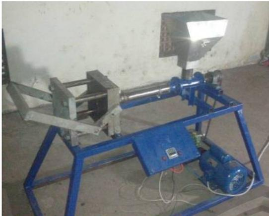
Gambar 4. Foto alat injection molding plastik
