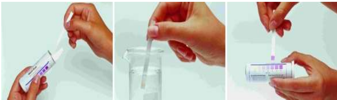
Gambar 2.6 Cara Penggunaan Test Strip (Sumber: www.merckmillipore.co.id/test-strip-merckoquant-/c_Y_Ob.s1Op00AAAE1A41tk03 )
