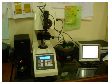
Gambar 5. Mikro Hardness Vickers merk TIME Beijing
