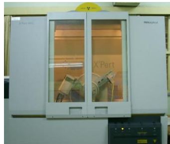
Gambar 2.12 Sistem High Resolution X-Ray Diffraction (HR-XRD) (Sumber: Laboratorium Geologi, Pusat Survei Geologi)
