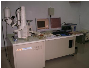
Gambar 2.15 Sistem Energy Dispersive X-Ray Spectrometer (EDS) (Sumber: Laboratorium Geologi, Pusat Survei Geologi).
