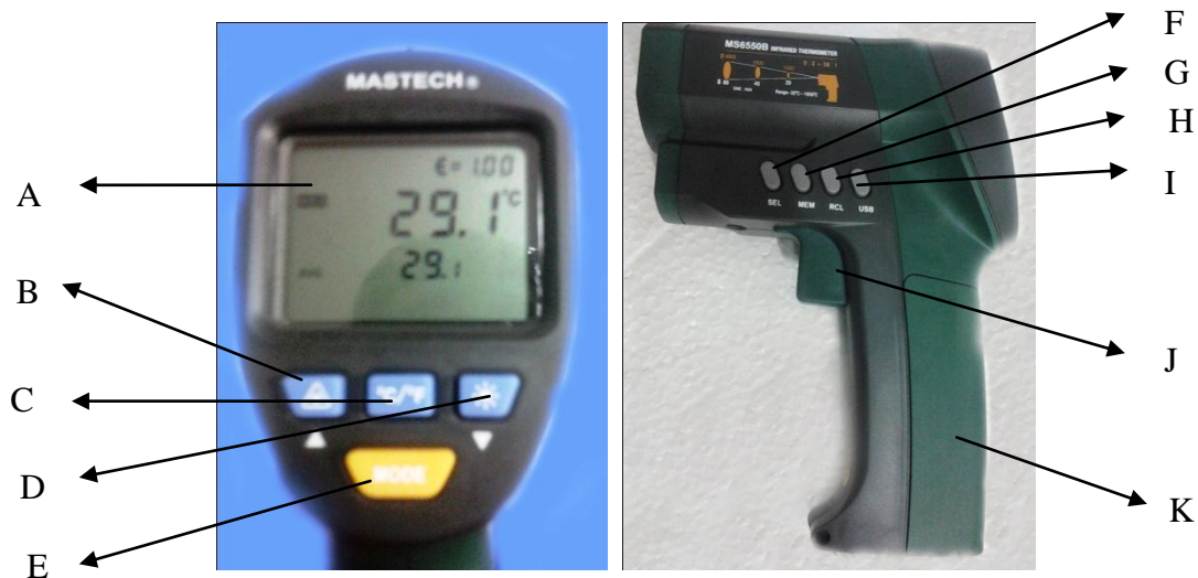
Gambar 3.3 Infrared Thermometer MS6550B MASTECH: (A) LCD, (B) Laser Key, (C) °C/°F Toggle Key, (D) Backlight Key, (E) Mode Selection Key, (F) Function Selection Key, (G) Save Key, (H) Recall Data Key, (I) USB Communication Key (J) Trigger, (K) Battery Cover.
