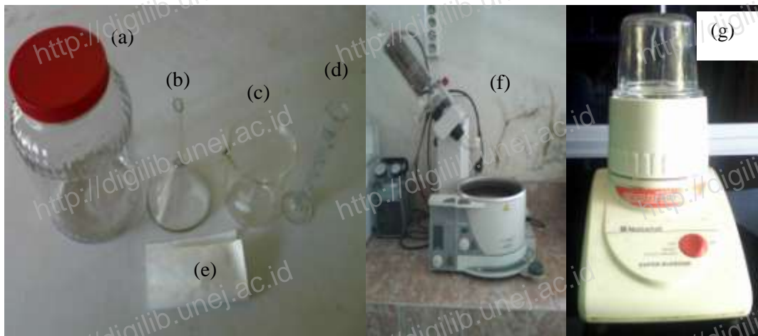
(a) Toples; (b) Corong Buchner; (c) Beaker glass ; (d) Gelas ukur; (e) Kertas saring; (f) Rotary evaporator ; (g) Blender
