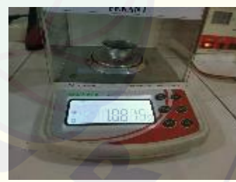
Pengukuran kadar abu
