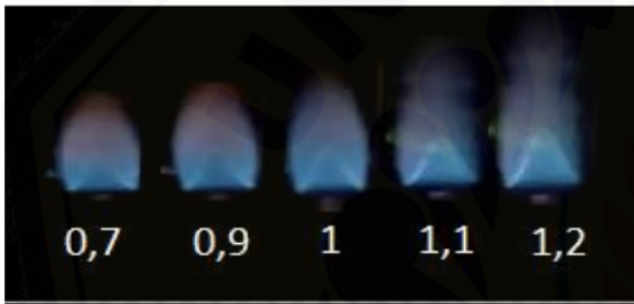
(b) ethanol flame with an equivalent ratio of 0.7-1.2
