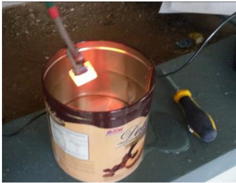
FIGURE 6. Quenching process of heated sample.
