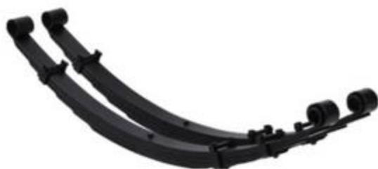
FIGURE 3. Leaf spring of a car.
