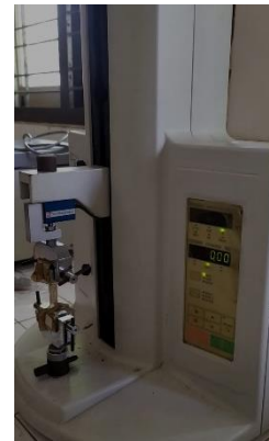
Fig. 8. The tensile test of biodegradable plastic
