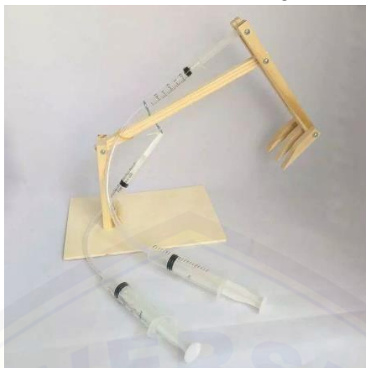
Figure 2. Simple Hydraulic Arm Instructional Aid
