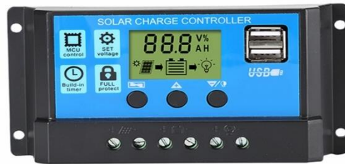
Gambar 2. 6 Solar charger controller
