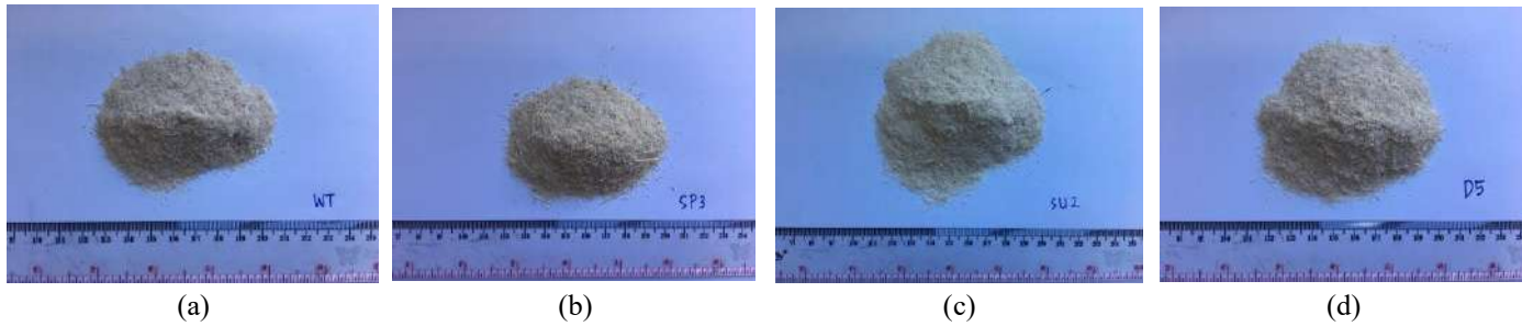
FIGURE 2. Sugar Cane bagasse that has been a grind with 50 Mesh particle size (a) Wild type, (b) PRG-SP3, (c) PRG-SU2, (d) PRG-D5.
