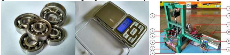
Figure 1. Rolling Resistance Test Equipment at Bearing
