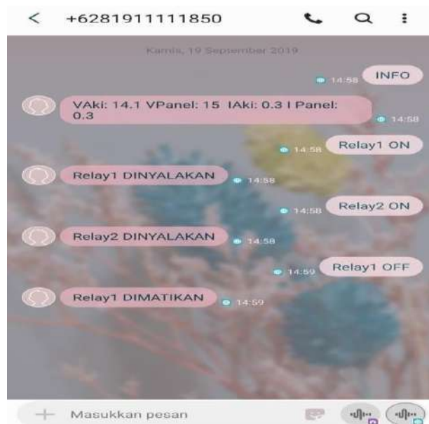
FIGURE 8. SMS commands to the tool and information from the tool
