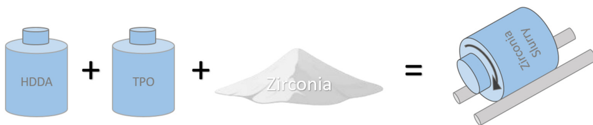
Figure 3. Preparation of making zirconia slurry.
